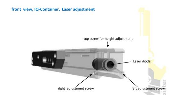
To be used only for adjustment of different target distances than 10 meters
